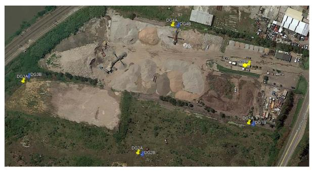
**Figure 2** Approximate Placement of Dust Deposition Gauges and Real Time Monitor.
