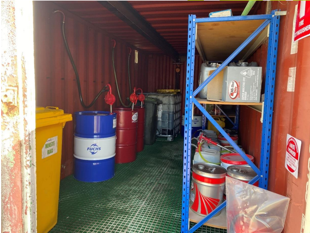
Photo 9 Hydrocarbons stored on bunds.
