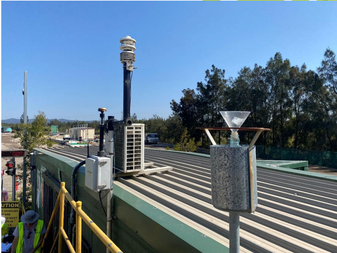
Photo 17 Depositional dust monitoring gauge and site air quality monitor.
