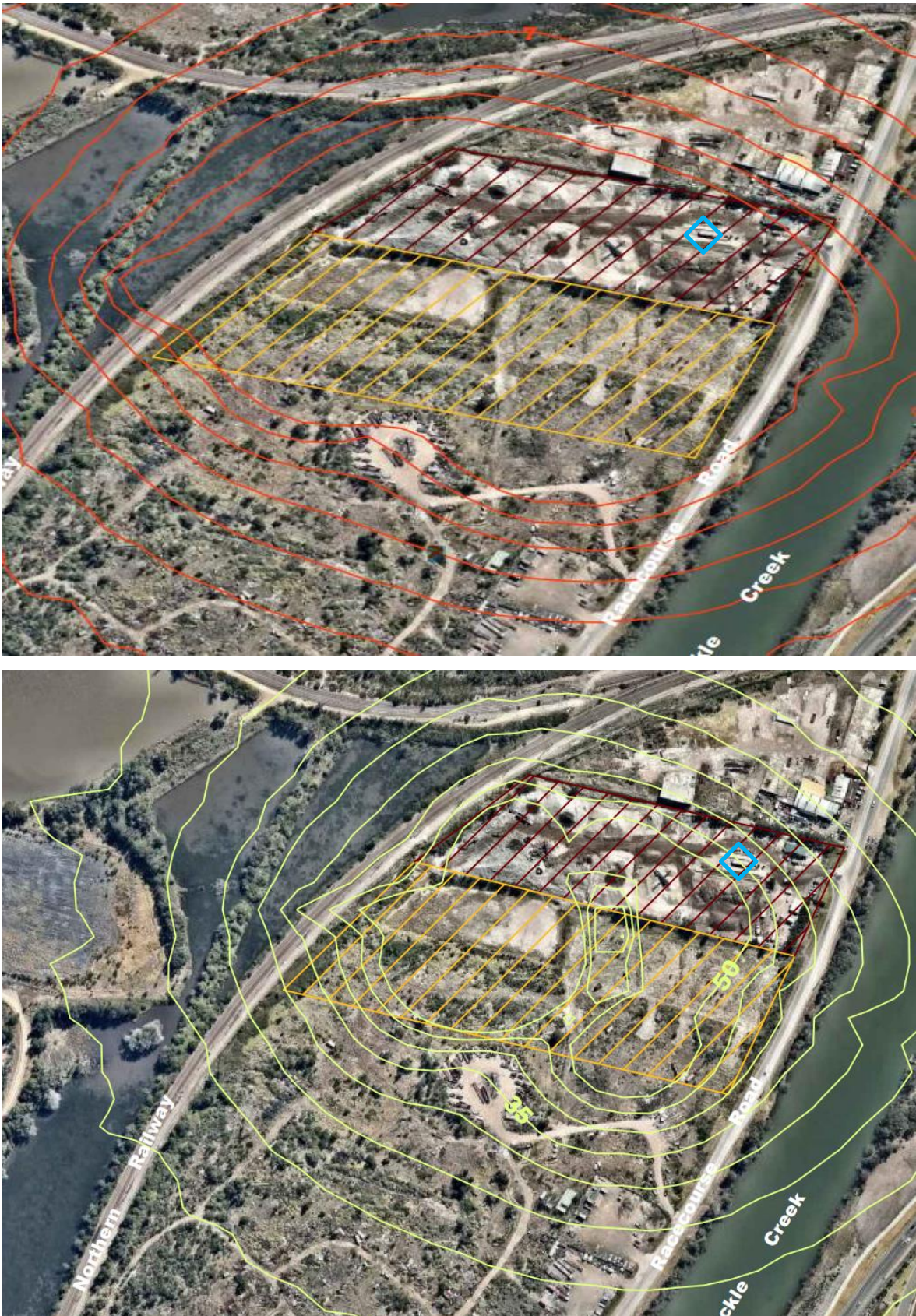
Figure 3 Predicted Daily PM 2.5 and PM 10 Impacts with Location of Real Time Dust Monitor Marked with Blue Diamond.
