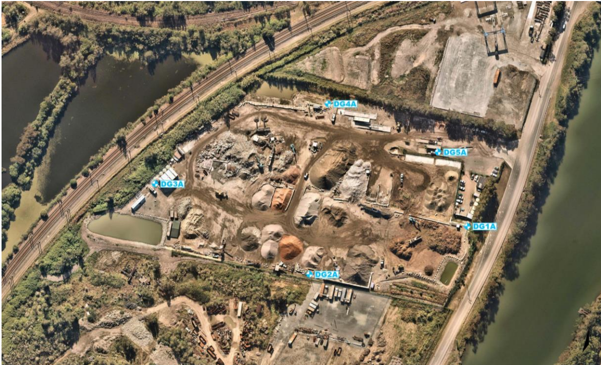
Figure 2 Approximate Placement of Dust Deposition Gauges and Real Time Monitor (aerial as of 23 May 2023).
