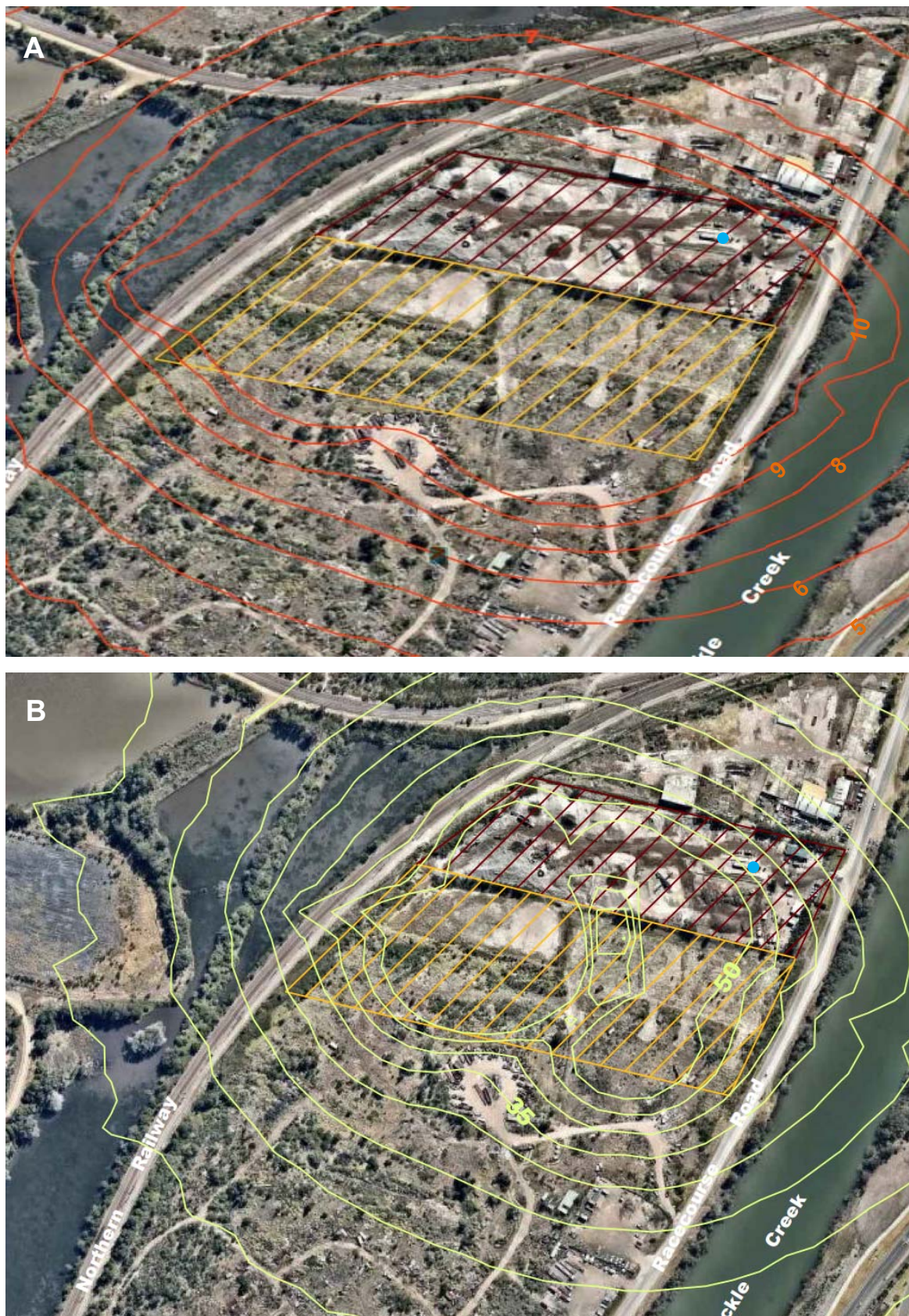
Figure 3 Predicted Daily PM 2.5 (A, top) and PM 10 (B, bottom) impacts with location of real time dust monitor marked with blue dot. All numbers are in units of \mu\text{g}/\text{m}^3 .
