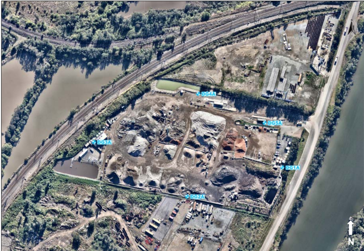
Figure 2 Approximate Placement of Dust Deposition Gauges and Real Time Monitor (aerial as of 26 June 2024).
