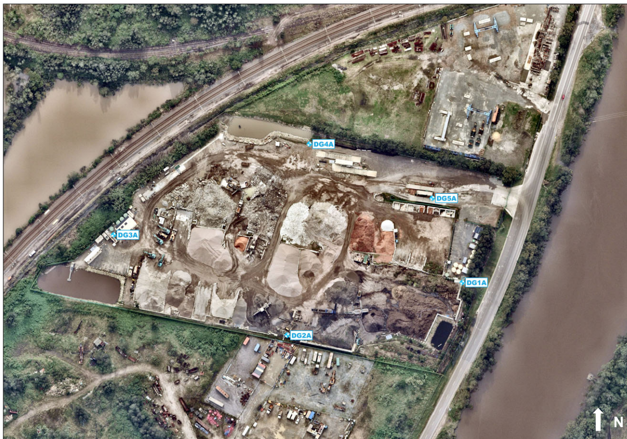
Figure 2 Approximate Placement of Dust Deposition Gauges and Real Time Monitor (aerial as of 25 May 2025).
