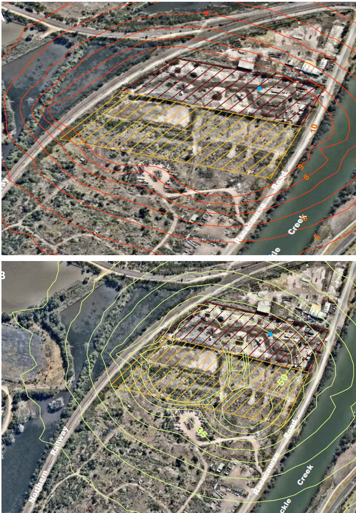
Figure 3 Predicted Daily PM_{2.5} (A, top) and PM_{10} (B, bottom) impacts with location of real time dust monitor marked with blue dot. All numbers are in units of \mu g/m^3 .
