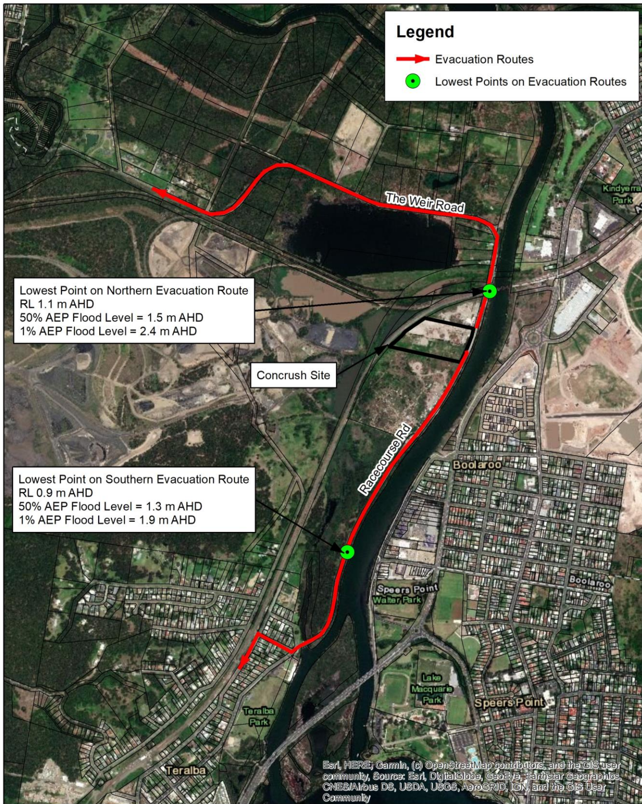
Figure 4.1 Evacuation Routes for Concrush Site
